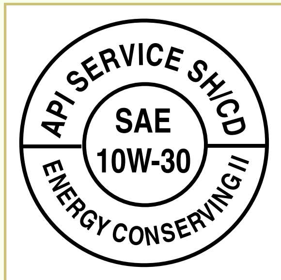
FIGURE 2 —All oils have labels showing a classification determined by the American Petroleum Institute (API) and the Society of Automotive Engineers (SAE) .
